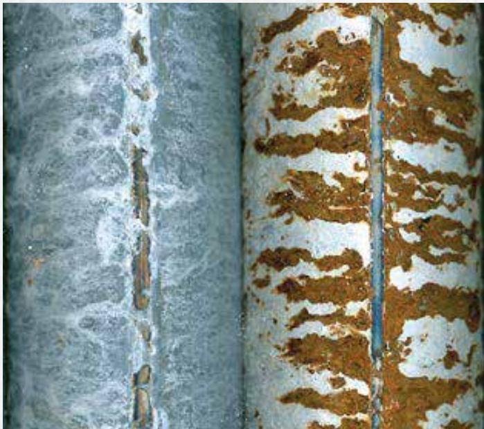
Magnelis® ZM120 welded, not re-protected
