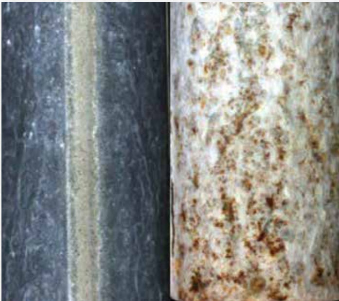
Magnelis® ZM310 welded and re-protected
